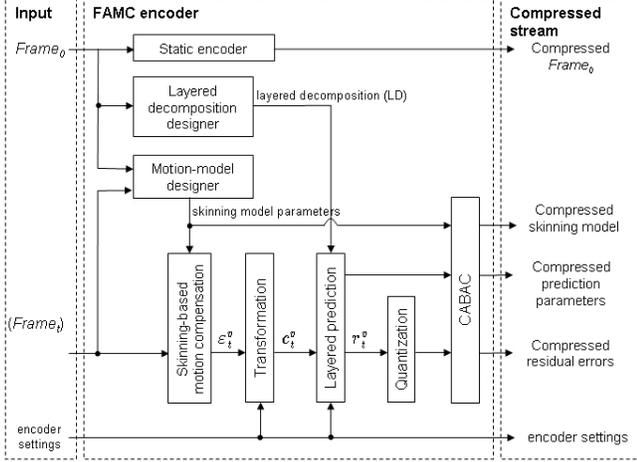
Fig. 1. Synopsis of the FAMC encoding algorithm.
